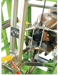
The only and unique system to firmly anchor the frames of motorcycles and scooters, thanks to universal jigs, columns adjustable in height and sliding crossbeams.
